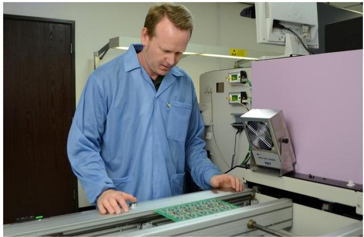
Also, ionizers are a much faster and more efficient method of neutralizing static charges on insulators/isolated conductors versus humidity control. The importance of air ionization cannot be understated as insulators/isolated conductors are now common at nearly every ESD workstation.
