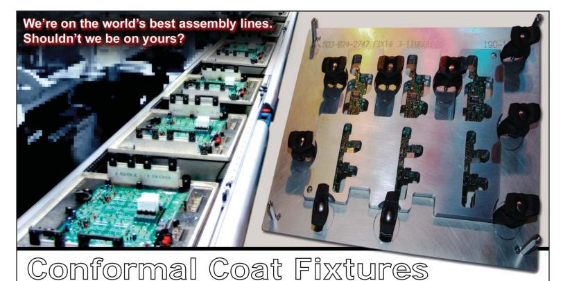
Pentagon's Conformal Coating Fixtures *save time* and provide *simple, fast, accurate and repeatable results* from your conformal coating masking operations. Just put the board in the fixture, close the covers, and you are ready to go. Conformal Coating Fixtures manufactured by Pentagon EMS are designed to support the PCB, yet maintain minimal contact with the PCB to ensure that coating buildup is minimized
