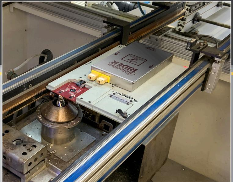
The SelectiveRIDER™ is a measurement pallet designed to capture parameters from the selective solder process and collect machine data for repeatability. It uses the SuperM.O.L.E.® Gold 2 profiler as the data collection device, and a dedicated environment in MAP software for analysis and SPC. It captures: fountain height, fountain X/Y accuracy, fountain diameter, solder temperature, maximum preheat, Delta T at contact, Flux penetration, and Fluxer X/Y accuracy.
