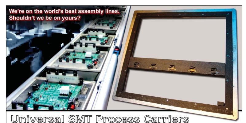
Process a wide variety of board shapes and sizes with a single fixture. Pentagon EMS
