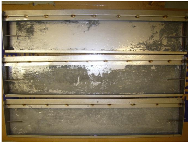
Figure 17: Solder Paste Collected in Sluice Boxes
