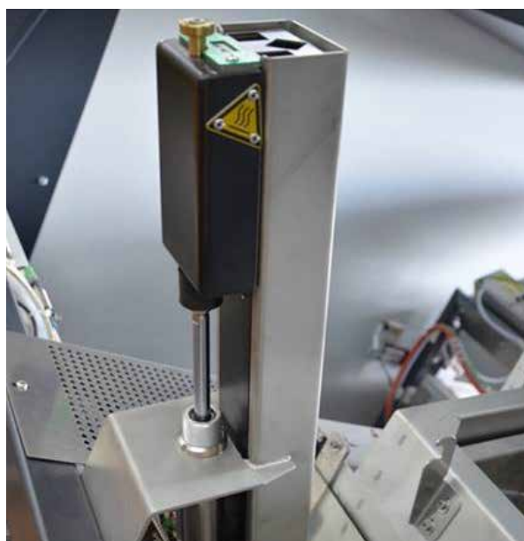
Automatic solder bar feeder
