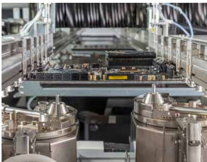
Dual pot system, Y- and Z axes variable
