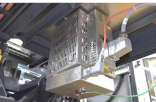
Electromagnetic solder pump
