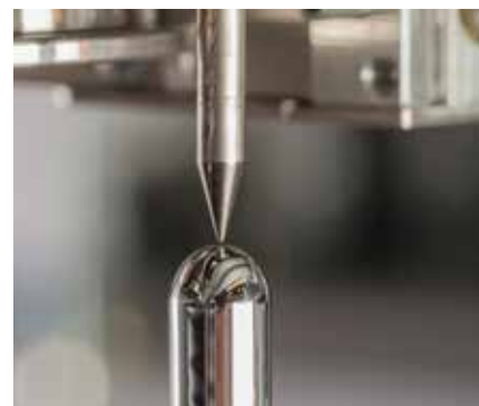
Automatic monitoring of solder wave height
