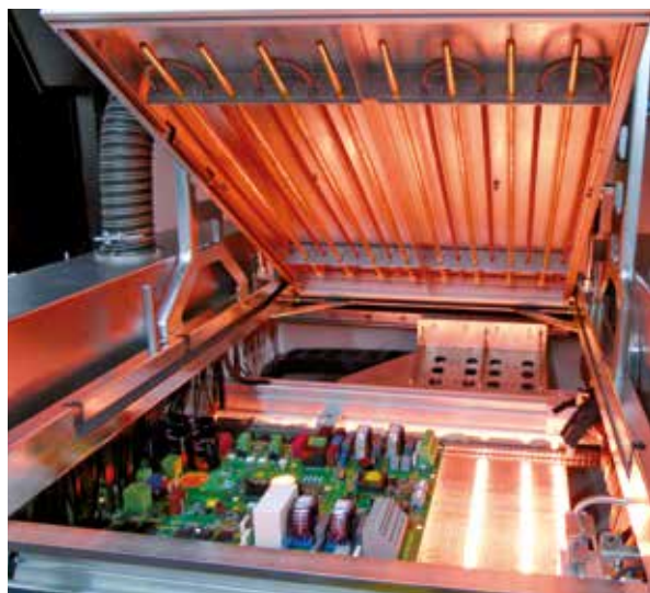
The Ersä preheat concept – a perfect combination of dynamic top- and bottom-side preheats with the venturi principle for reproducible results
