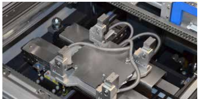
Fluxer unit with 4 spray heads
