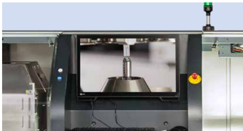
Visual process control – camera system shows real-time soldering process and assists in detecting defects
