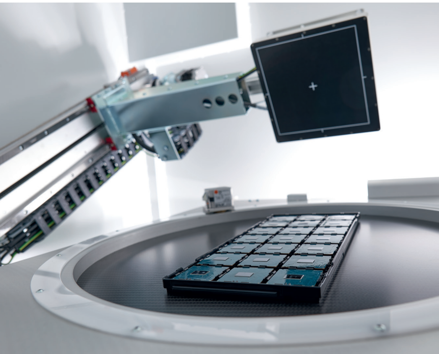
Automated 3D laminography inspection for maximum productivity.
