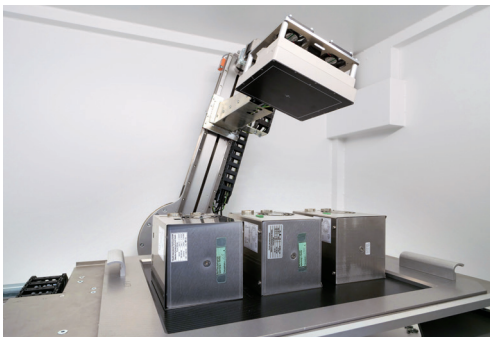
The high load option of Cheetah EVO is suitable for parts with a weight of up to 20 kg.
