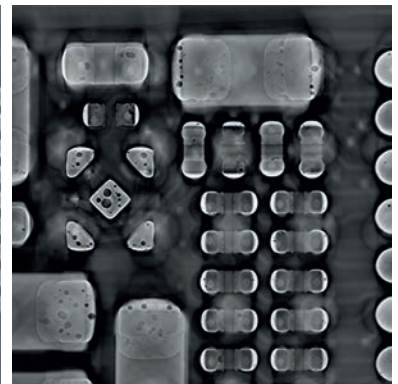
LayerScan (Vista X Pro): resolution 0.9 \mu\text{m} , 12 min scan time.
