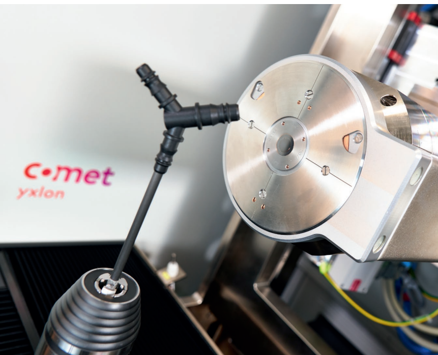
The FF20 CT's 190 kV nanofocus transmission tube delivers high detail visibility.
