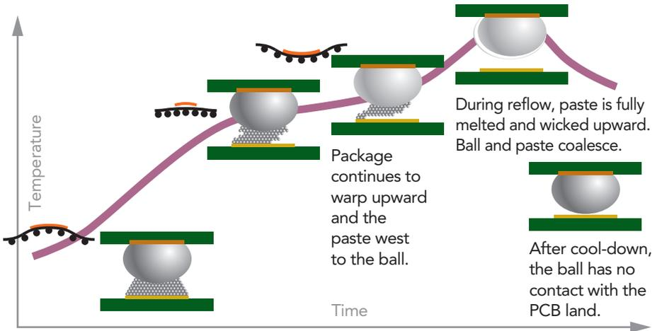
Solder paste preferentially wets to the solder ball rather than the PCB land. Mechanism primarily driven by paste characteristics.
