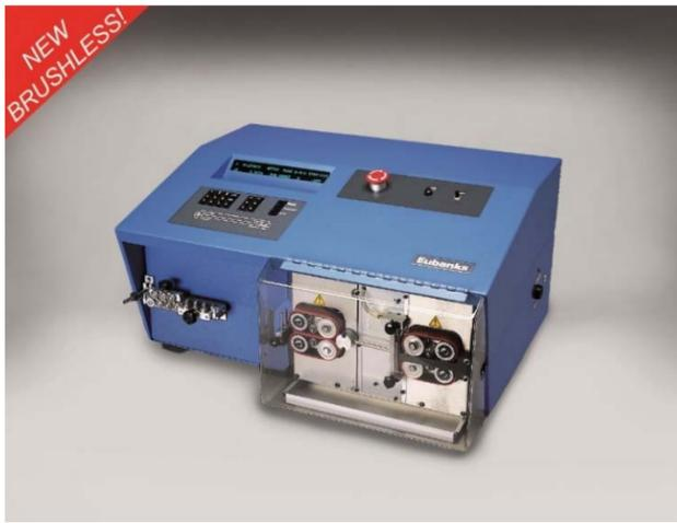
The new Model 7600 is as rugged and powerful as the model 8900. It covers a complete range of wire sizes from 32 through 6 AWG thin-stranded wires. If you are searching for a reliable wire processor that will serve for years and your production needs are from small to medium size wires, the 7600 excels at this range, doing either high-mix & low-volume or high-volume, low-mix.
