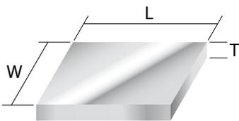
**ALPHA AccuFlux BTC-578 Preforms** are sized to support the most common bottom terminated component packages (QFN, QFP, D-PAK, etc.) to optimize void reduction.
