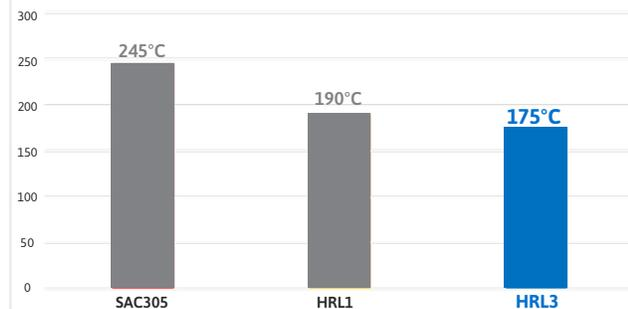
HRL3 Alloy Enables Target Peak Reflow 175°C
