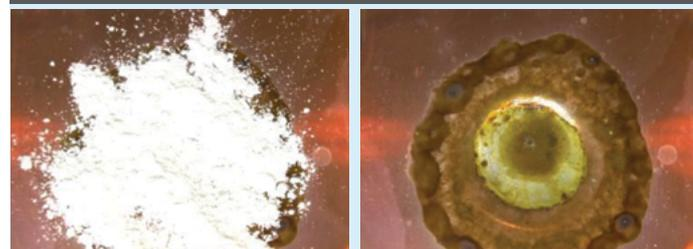
Tack test result shows that ALPHA EF-8800HF residue is non-tacky.
